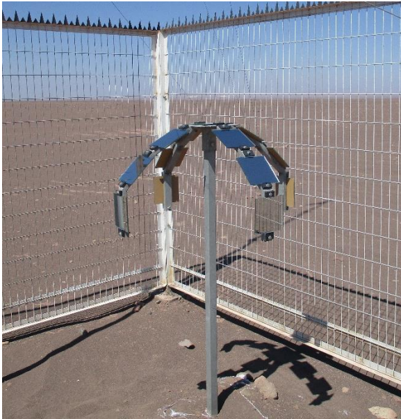
Spider structure to position mirrors to be studied in multiple orientations and angles
