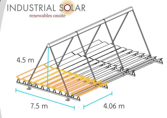
Generates heat up to 400 °C and 120 bar
