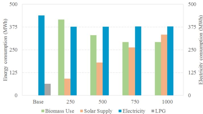
Fig. 3. Solar, biomass and electricity use in summer for the base case and different collector field areas
