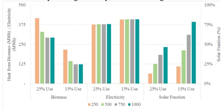
Fig. 5. Comparison of 15% and 25% usage of the absorption chiller.
