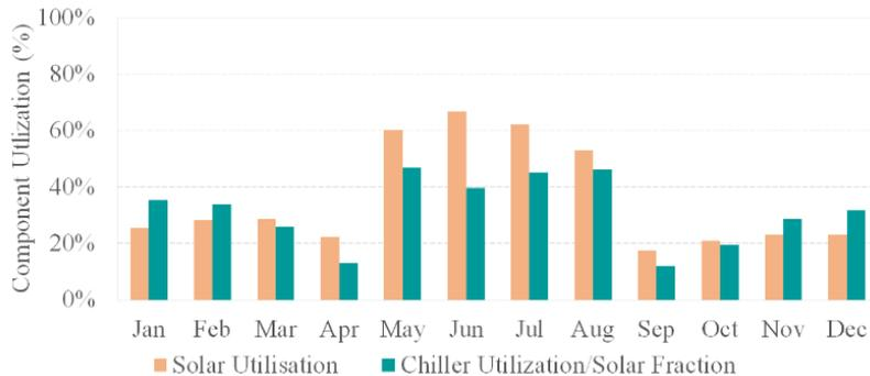
Fig. 8. Monthly performance of solar and chiller utilisation and solar fraction for 500m<sup>2</sup>
