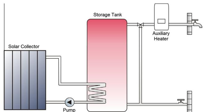
Fig. 9. Solar system configuration for residential water consumption scenario.
