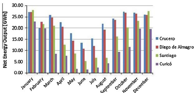
Fig. 12. Monthly net energy output of a parabolic trough plant for the selected locations.
