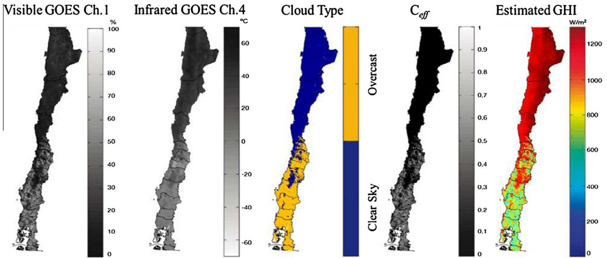
Fig. 5. Summarized procedure of the Chile-SR model: from visible and IR satellite images to estimated GHI.
