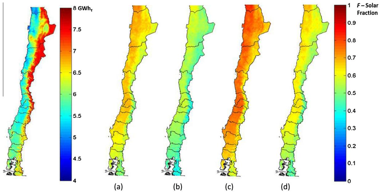
Fig. 10. Annual energy load for residential water heating, as function of the geographic location, in GW h (left), and annual solar fraction using (a) high performance; (b) low performance flat plate solar collectors; (c) high performance, (d) low performance evacuated tube collector.
