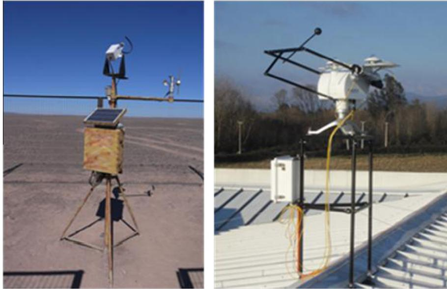
Fig. 2. RSBR station in Crucero and one station with tracker, pyrheliometer, and pyranometers in Talca.
