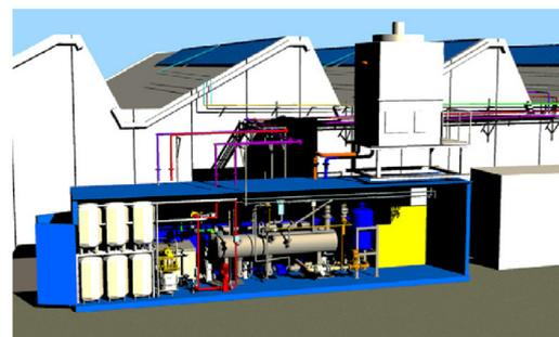
Fig. 19. Technical drawing of the steam generation unit (left) and pilot plant (right) (Joemann et al., 2016).
