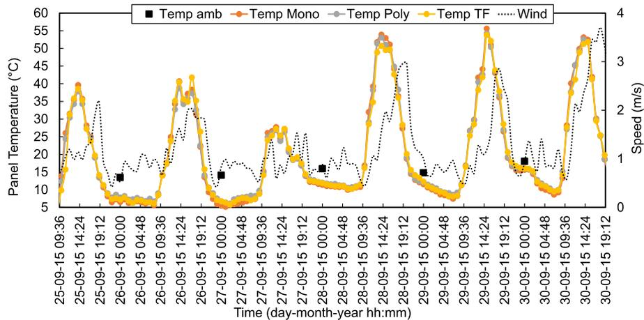
**Fig. 3.** Temperature of solar panels and wind speed for 6 days of analysis.
