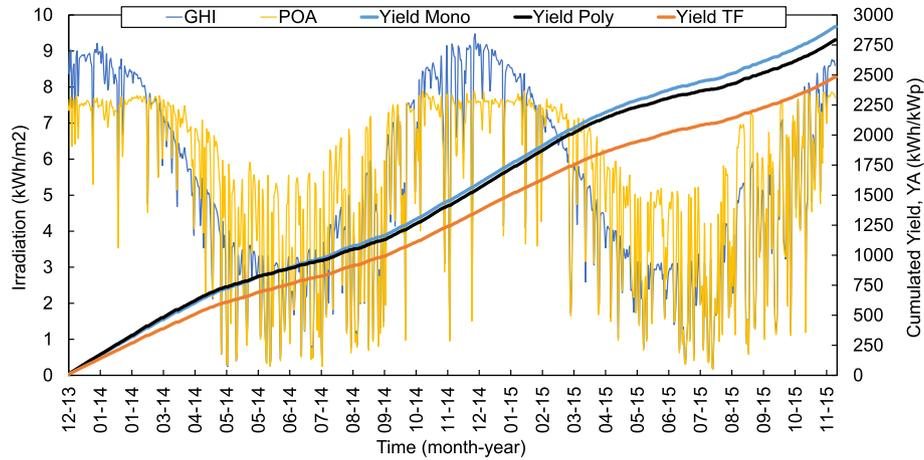
**Fig. 2.** Two years data for global irradiation *POA* and *GHI* in Santiago (Chile) and cumulated final yield of array,  $Y_A$ , for all PV technologies.  $32^\circ$  tilt angle and  $350^\circ$  azimuth, shifted  $10^\circ$  towards the West.
