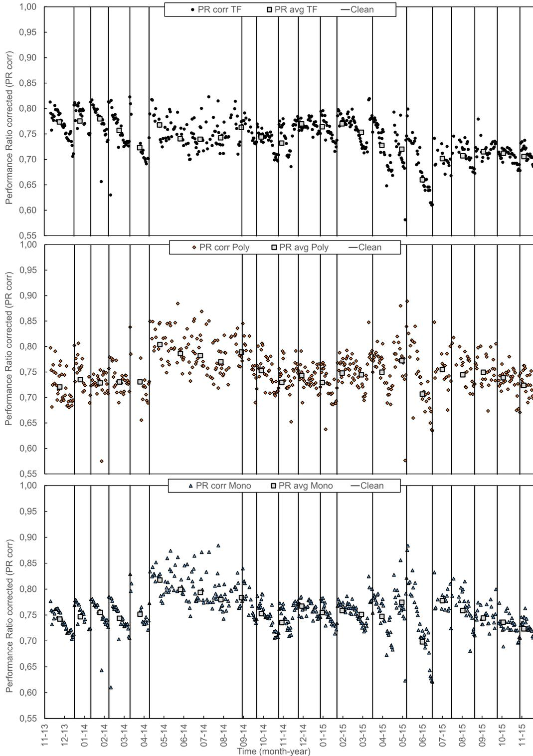
**Fig. 5.** Weather-corrected performance ratio in two years period December 2013 – November 2015, for TF, Poly and Mono PV arrays, respectively. Monthly cleaning is shown in full vertical lines. The time line is shown in the bottom x-axis in month-year format.
