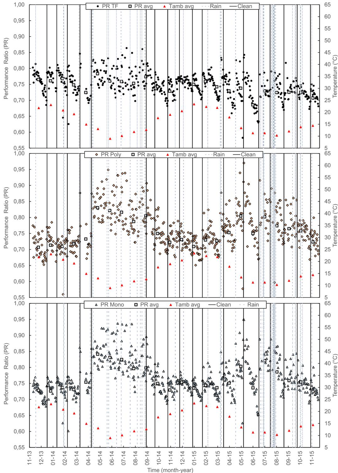
Fig. 4. Average daily and monthly PR for TF, Poly, and Mono PV arrays and average monthly ambient temperature  $T_{amb}$ , measured within two years period: December 2013 – November 2015. Monthly cleaning and rainy days are shown in full and dashed vertical lines, respectively. The time line is shown in the bottom x-axis in month-year format.
