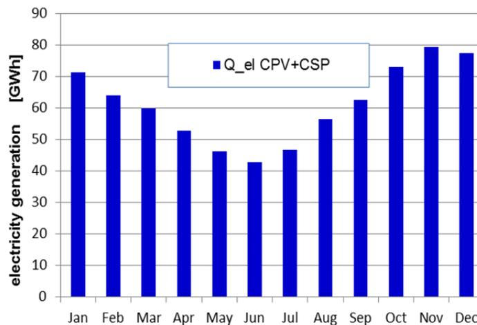
**FIGURE 6:** Monthly electricity production by combined CSP-CPV power plant 100 MW<sub>e</sub> for Upington, South Africa; (150 MW CPV, 15h TES, Solar field SM 2.2)
