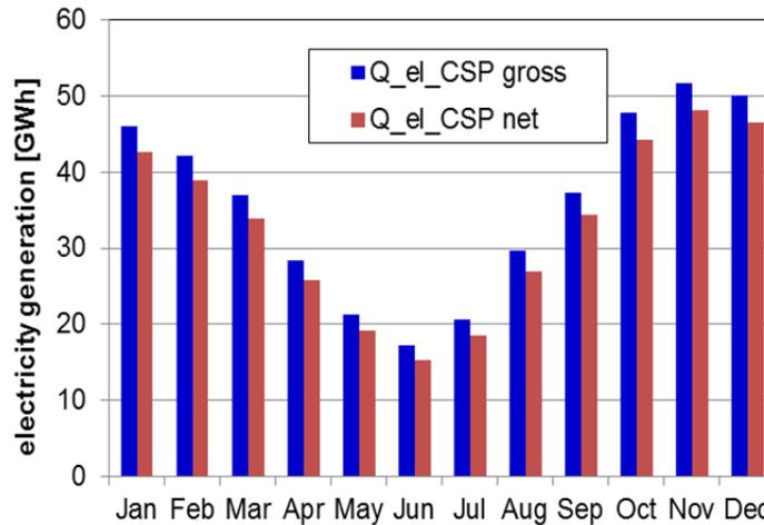
FIGURE 4: Monthly electricity generation (gross and net) for the LFC plant with SM=2.78 and 9h TES
