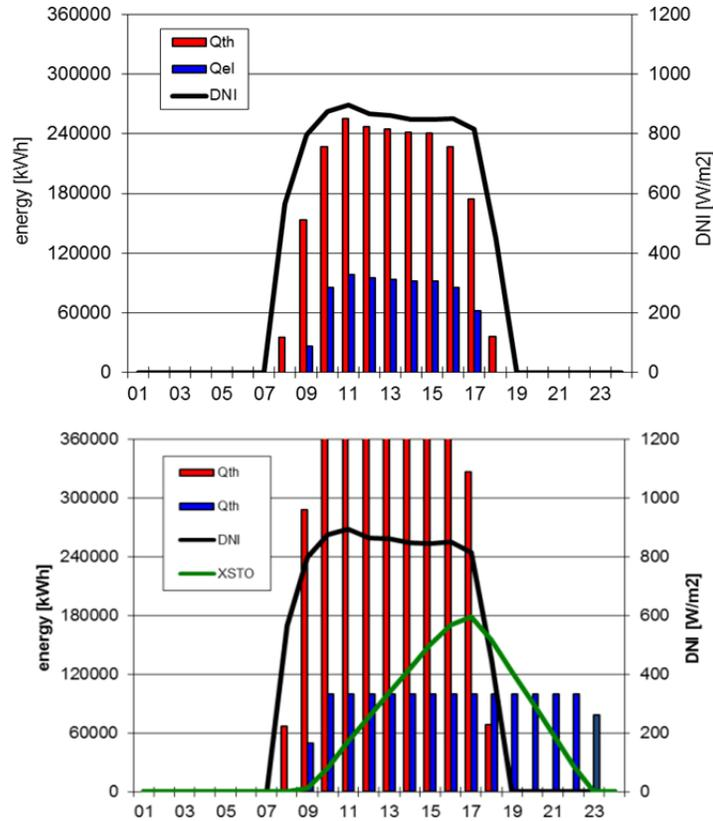
**FIGURE 3:** Hourly DNI (black), produced thermal energy  $Q_{th}$  (red) and generated electricity  $Q_{el}$  (blue) for the case  $SM=1.48$  w/o TES (top) and  $SM=2.78$  with 9h TES (bottom); the green curve XSTO shows the filling level of the hot storage (1000 on the right axis equivalent to 100%)
