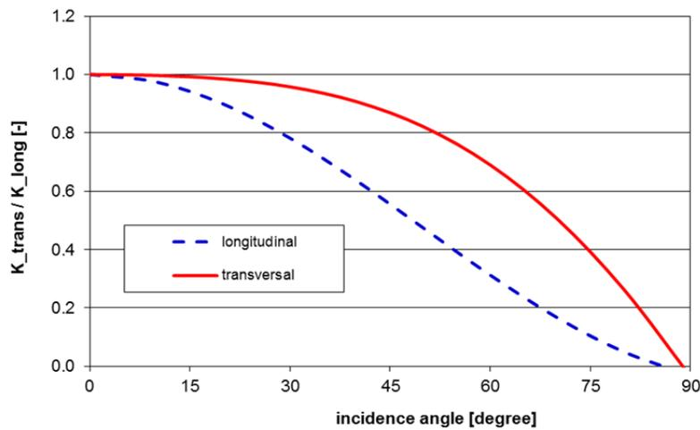
**FIGURE 1:** Longitudinal and transversal incidence angle modifier for the generic Linear Fresnel Collector
