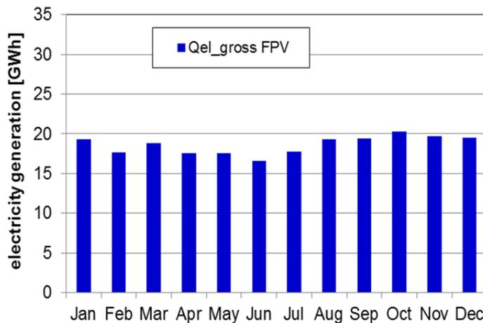
FIGURE 5: Monthly electricity generation for a 100 MW FPV plant, Uptington, South Africa
