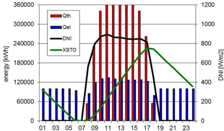
**FIGURE 7:** Hourly electricity production by combined CSP-CPV power plant 100 MW<sub>e</sub>
