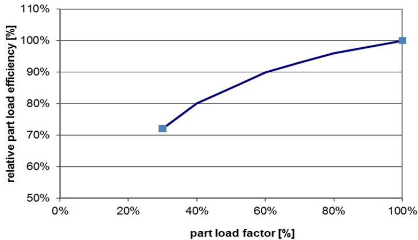
**FIGURE 2:** Factor for turbine efficiency at part load between 30% and 100% nominal load
